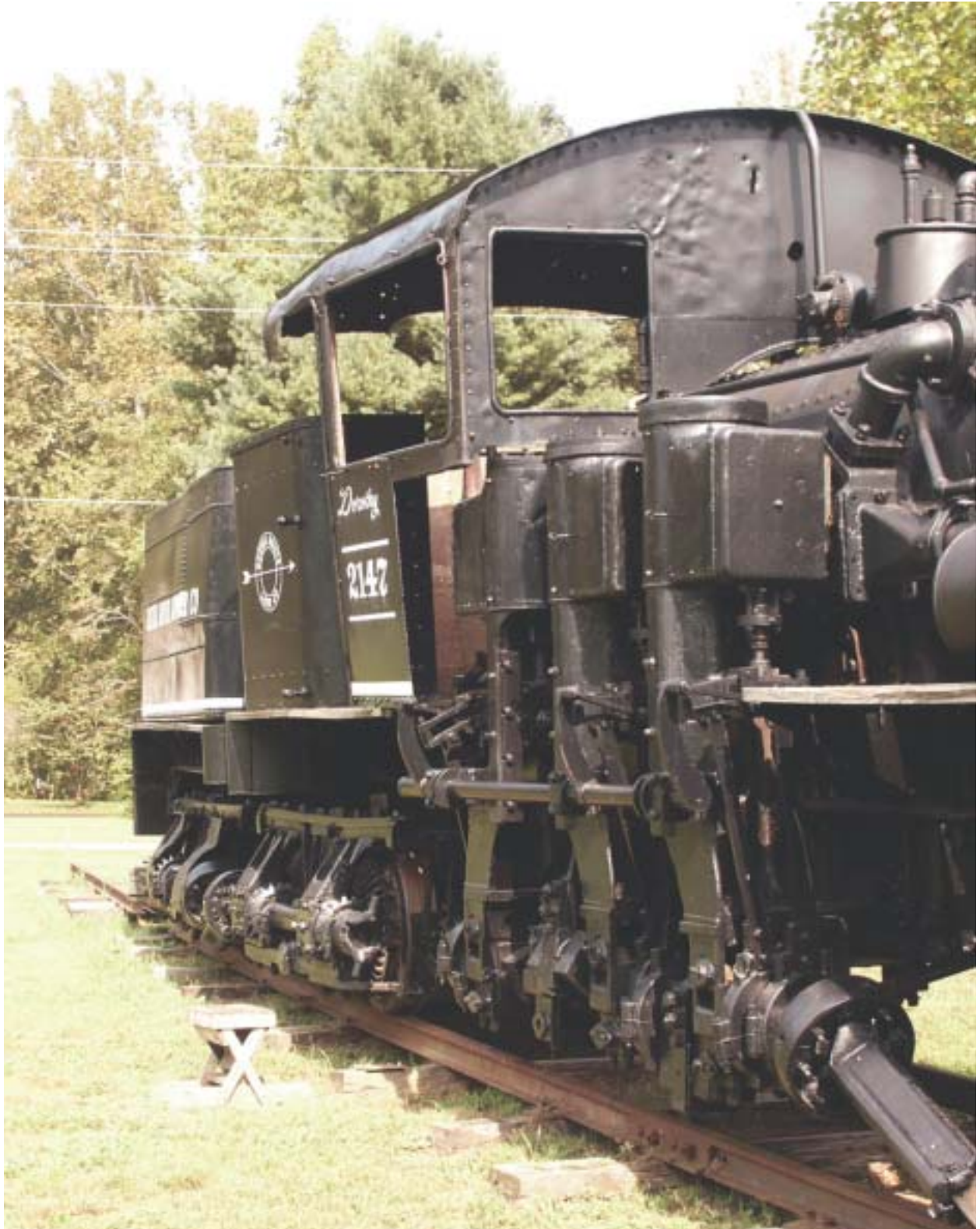
An unusual but powerful drive mechanism of a mountain locomotive
